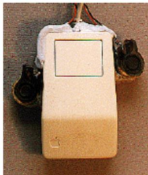
Figure 5: Stereo Vibrotactile Mouse
