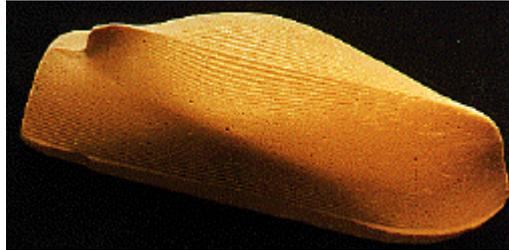
Figure 3: Ship Hull Example: 3D hard copy revealed lack of fairness at bow and stern when touched
