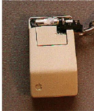
Figure 6: Mono Solenoid Mouse
